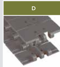
HP 820 Series PITCH: 1.5-inch (38.1mm) THICKNESS: 0.15-inch (4.0mm) For high-speed single file vacuum conveyors
